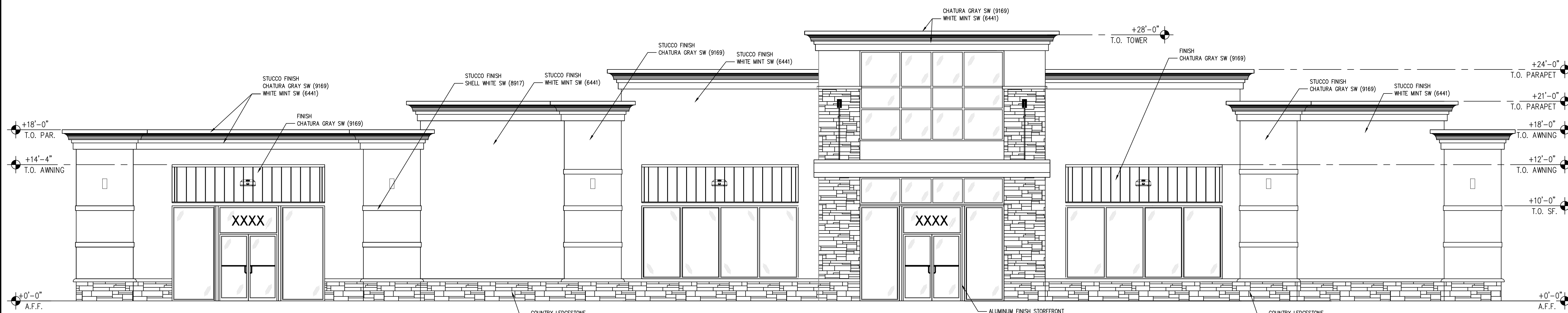
1 FRONT ELEVATION SCALE: 3/16" = 1'-0"
